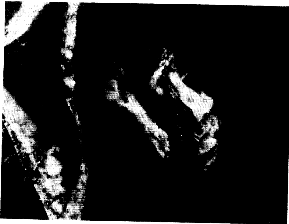
Photograph 18: Paper fiber standard showing cellulose fiber with clay sizing. The photograph was taken using polarizing filters 15 degrees off crossed. 320x magnification.
