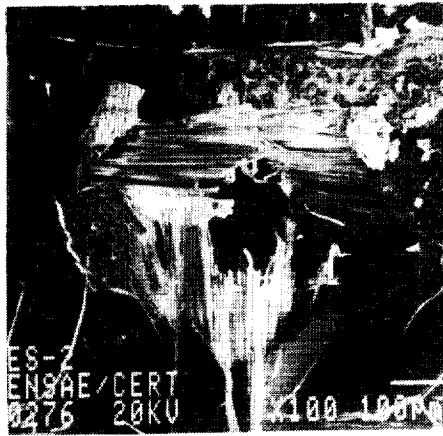
Fig.4. This figure shows a typical crater on tefloned fiber glass fabric.
