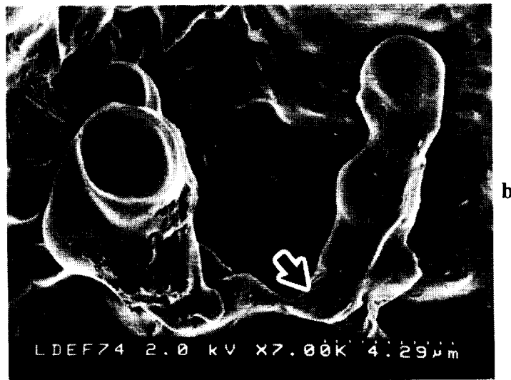
Figure 3. (a) Melt splash on the wall of crater #74. (b) Partially melted impactor grains that are coated with glass. Arrow points to twisted, pinched glass. (FESEM BSE image).
