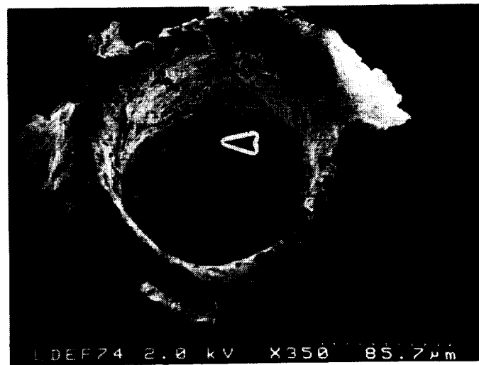
Figure 1. (a) FESEM BSE (backscattered electron) image of crater #74. Arrow points to round residual grain which is used as a reference in other figures. Fractures in Al that radiate away from the crater (NW direction), probably resulted from ductile/brittle fracturing during uplifting of the rim. Carbonaceous material (dark; curved arrow) is shown on the top of the overturned, raised rim. (b) Same crater as in (a) (slightly tilted and rotated 180°). FESEM BSE image. Note partially intact residual impactor in the crater bottom. 10 division scale is given in microns in the lower right corner of all FESEM images.
