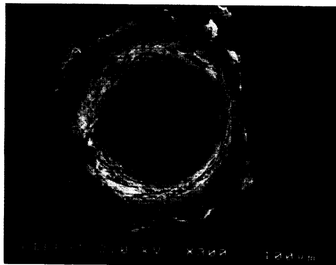
Figure 5. Crater #31. Impactor residue is probably all glass. (FESEM BSE image).
