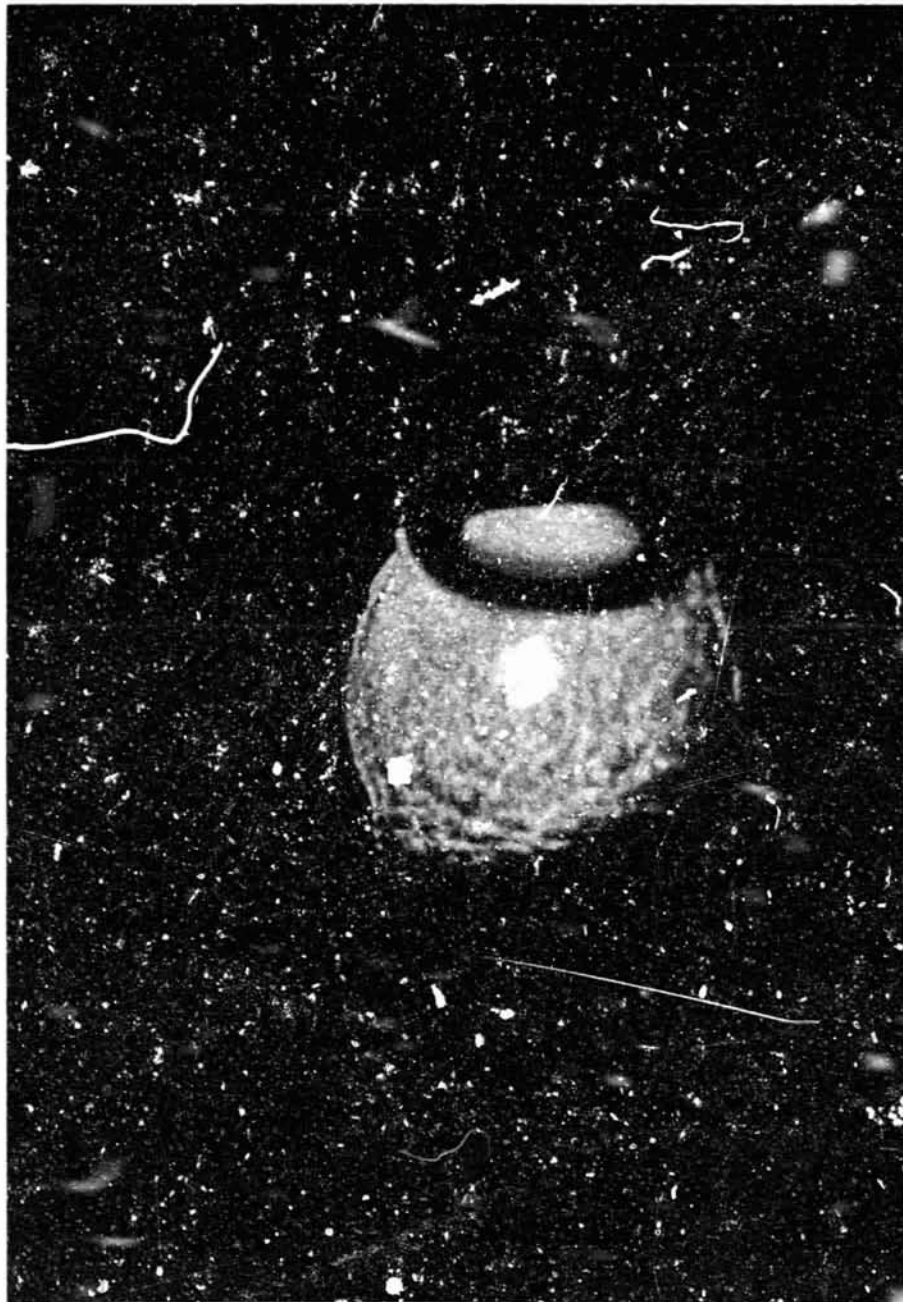
Figure 2. Binary fluid mixture of methanol-deuterated cyclohexane being mixed by ultrasounds with the CPF during ground tests. An air bubble can be seen at the top. The white dot in the middle is the thin laser beam used for scattering diagnostics.
