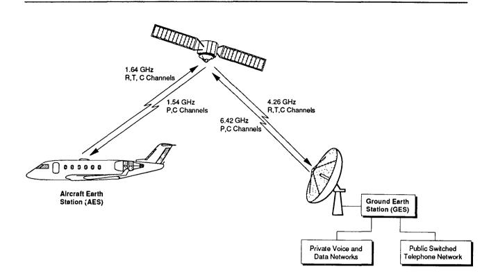
Figure 1 GA System Architecture
