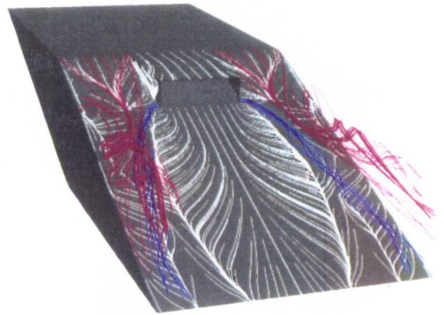
Figure 9. Simulated surface oil flow pattern and particle traces for the model with side extensions.
