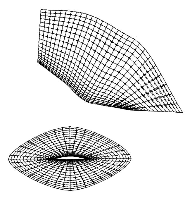
Figure 4. A comparison of 3D Bézier grids (solid lines) and transfinite interpolation grids (dash lines).
