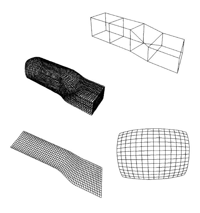
Figure 1. Wire frame and surface grids for a duct with a varying cross section.
