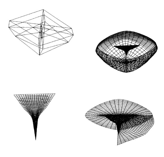
Figure 3. Wire frame and surface grids for a high speed aircraft.
