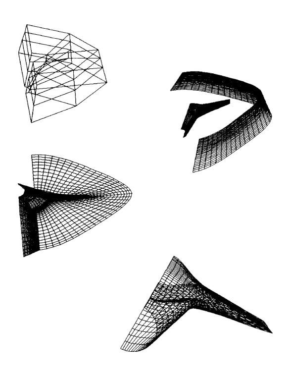
Figure 2. Wire frame and surface grids for a wing and part of a fuselage.
