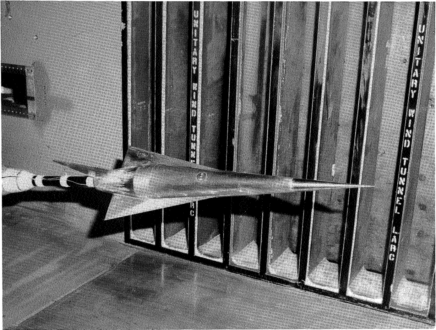
Figure 2 Photograph of model mounted in test section 2 of Unitary Plan Wind Tunnel, W1BN5V1 configuration
