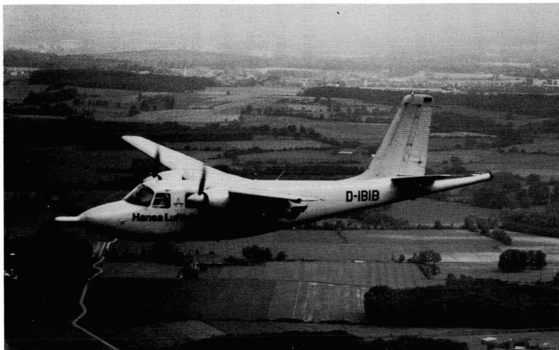
Figure 1. Aero Commander aircraft equipped for aeromagnetic and VLF electromagnetic surveys.
