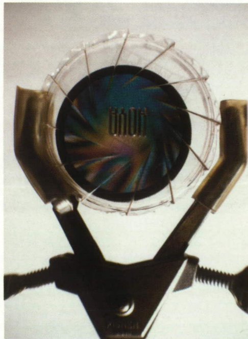
Plate 19. This polarizing filter enclosed within a birefringent plastic case was photographed under tungsten illumination with a polarizing filter on the camera. The colors are purer and span a wider gamut than those shown in Plate 17 because tungsten light is redder than skylight and the degree of polarization of the light incident on the case is higher than that of skylight.
