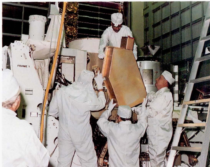
Technicians at Kennedy Space Center integrate the SUSIM instrument with the OSS-1 payload.
