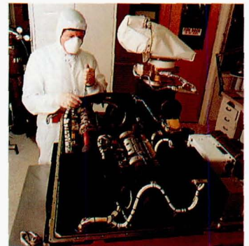
The ATMOS instrument's intricate optical equipment is checked during this preflight inspection.
