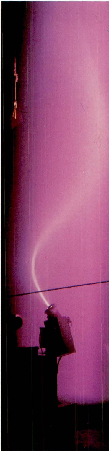
Enclosed by walls in a laboratory on Earth, an electron beam spirals around magnetic field lines and ionizes nitrogen gas, causing the purple glow. In like manner, scientists will inject electron beams into the atmosphere to learn how particles move through plasma.
