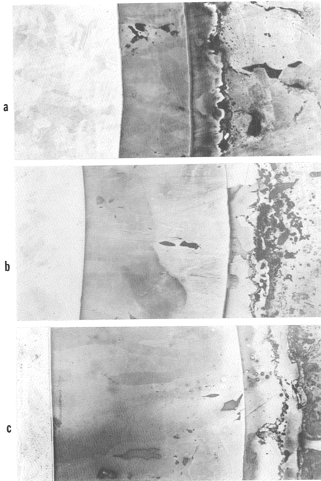
Figure 1. Single-phase layers in the Cu-Zn diffusion couples held at 400° C for (a) 1 day, (b) 4 days, (c) 9 days. Mag. 50x.
