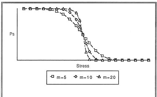
Figure 3: How probability of survival changes with Weibull modulus. Note that for higher values of Weibull modulus, there is less variation in fracture strength from specimen to specimen.
