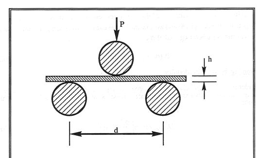
Figure 4: A rectangular specimen under a load P in a three-point bend test. The portion of the specimen under a tensile load has a length d, a thickness h/2, and a width w.
