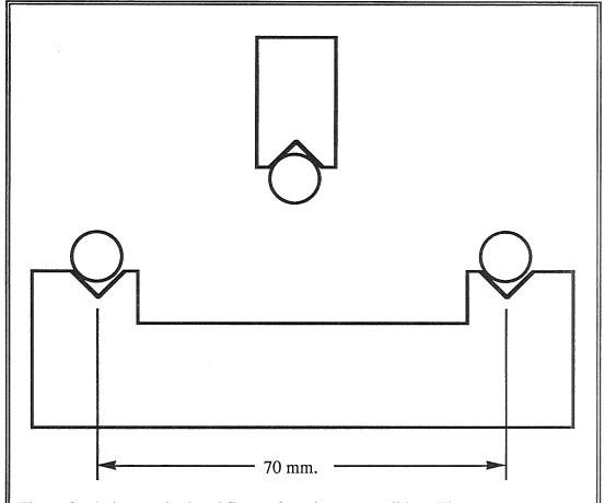
Figure 2: A three-point bend fixture for microscope slides. The support bars may simply be placed in the v-groove; the top force bar should be screwed to its support. The only critical feature of the construction is that the bars must be parallel.
