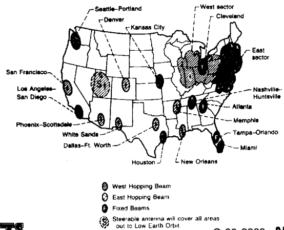
Figure 4.—Geographical coverage of ACTS Multibeam Antenna - example of steerable antenna beam also shown. Polarizations indicated are uplink. Downlink polarizations are opposite.
