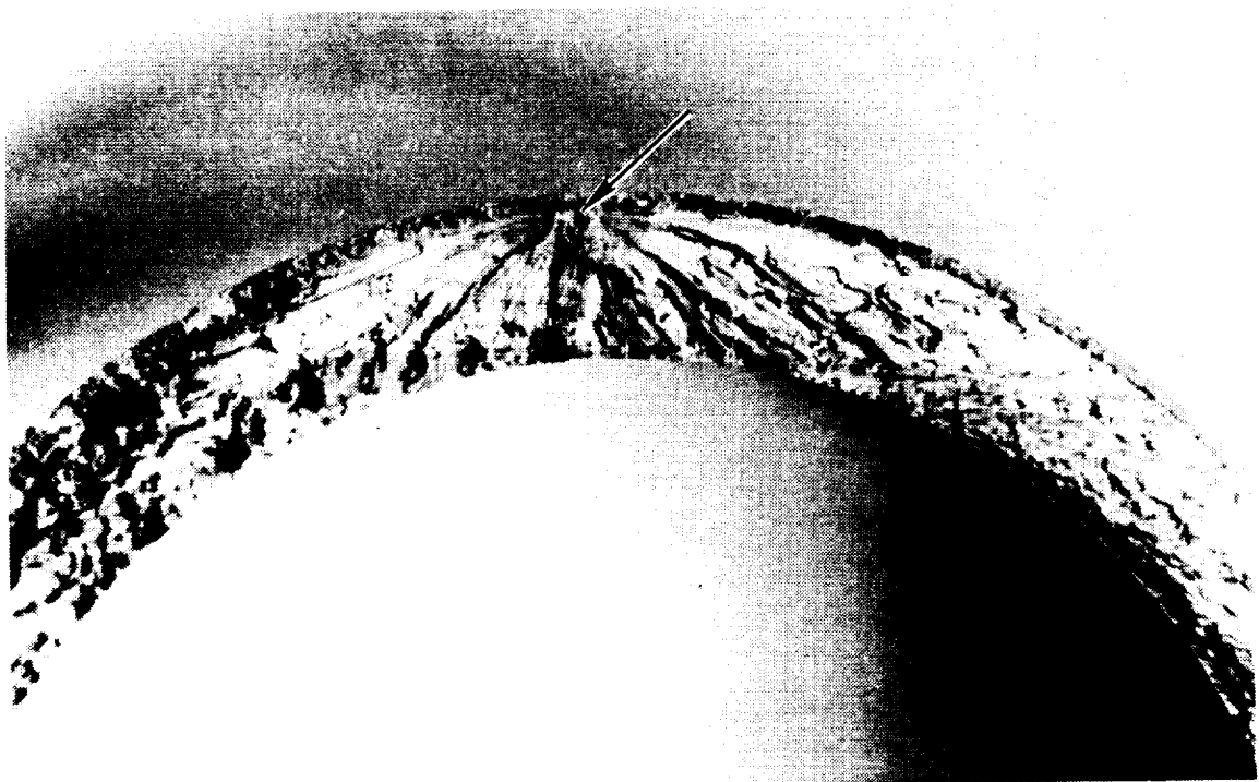
Figure 43 Optical Microscopy Image of PWA 286 Overlay Coated \langle 011 \rangle PWA 1480 Specimen KB-65 After Isothermal LCF Testing At 927°C (1700°F), \pm 0.25\% , 1 cpm for 6624 cycles. Arrow indicates location of subsurface PWA 1480 porosity where crack initiation occurred.
