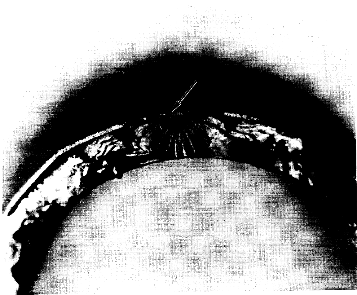
Figure 45 Optical Microscopy Image of PWA 286 Overlay Coated \langle 111 \rangle PWA 1480 Specimen LB-181 After Out-of-Phase TMF Testing At 427-1038^{\circ}\text{C} ( 800-1900^{\circ}\text{F} ), \pm 0.125\% , 1 cpm for 7675 Cycles. Arrow indicates typical coating initiated crack.
