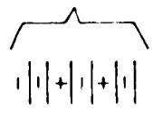
(o) Case 8, Balance yawed 180° and rolled 90° counterclockwise (reversed and rolled 90° counterclockwise) or pitched 180° and rolled 90° clockwise.
