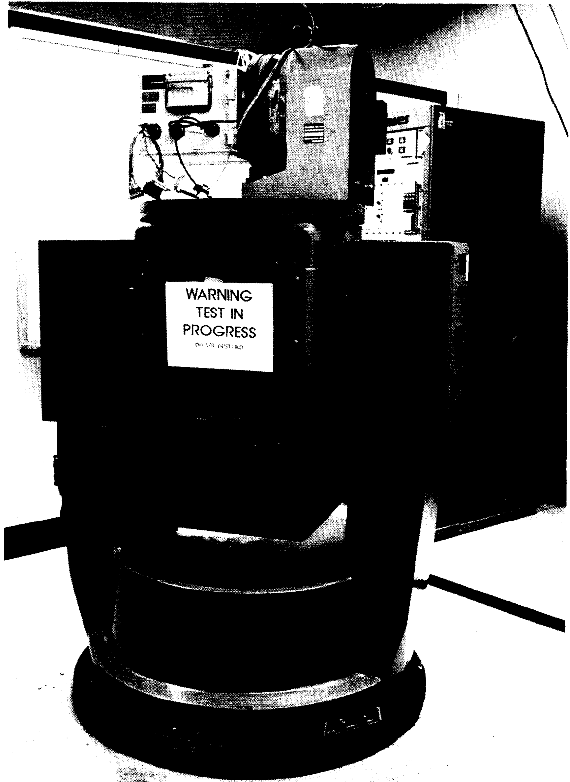
A front view of the air-bearing table and its control console. The table is installed on an isolation pad to isolate any building vibrations.
