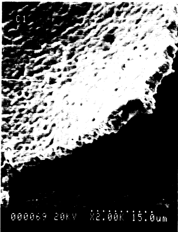
Figure 3.2.2-4. Uncoated NASA-Z Cylinder After Oxidation and Test – Center Area (>2.7% Strain)
