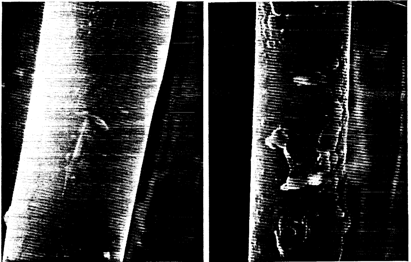
Figure 11. Scanning electron microscopy of non-coated fibers. (a) SiC as-received fiber, (b) SiC fiber exposed at 1200°C for 10 min.
