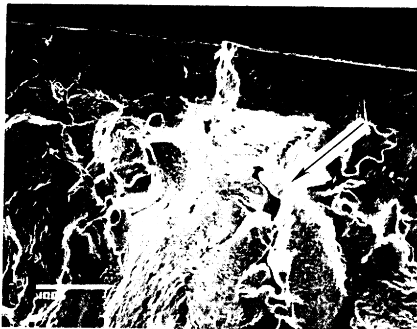
Figure 39 Secondary Electron Image of PWA 273 Aluminide Coated \langle 111 \rangle PWA 1480 Specimen LB-124 After Isothermal LCF Testing At 760^{\circ}\text{C} ( 1400^{\circ}\text{F} ), \pm 0.3\% , 0.5 cpm for 1372 cycles. Arrow indicates location of subsurface PWA 1480 porosity where crack initiation occurred.
