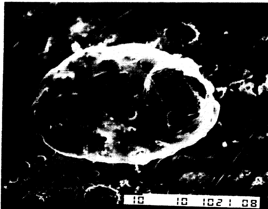
Fig. 16 Aluminum Ejecta Particles with Associated Splash Patterns
