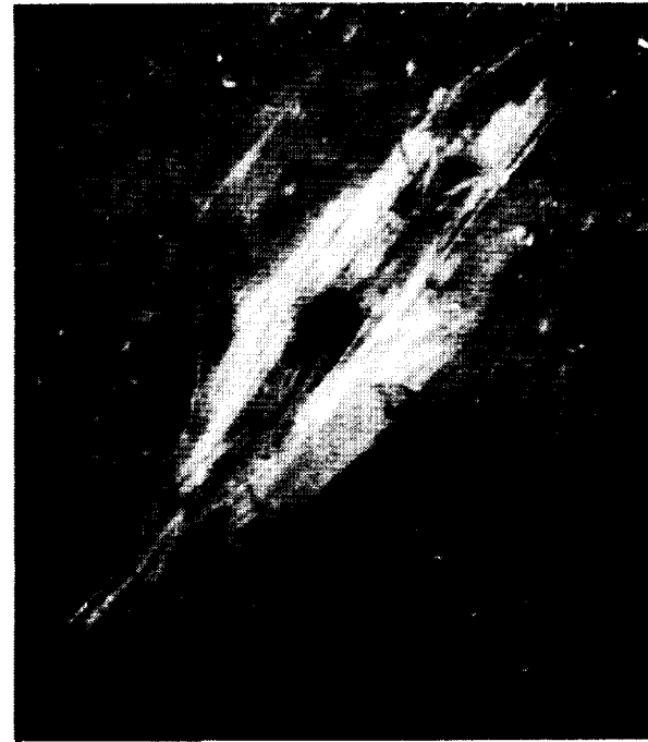
Fig. 19 Micrometeoroid/Debris Impact Damage (x100) on Kevlar®/Epoxy Tube [SP-328, (\pm 45^\circ)_{4S} ]
