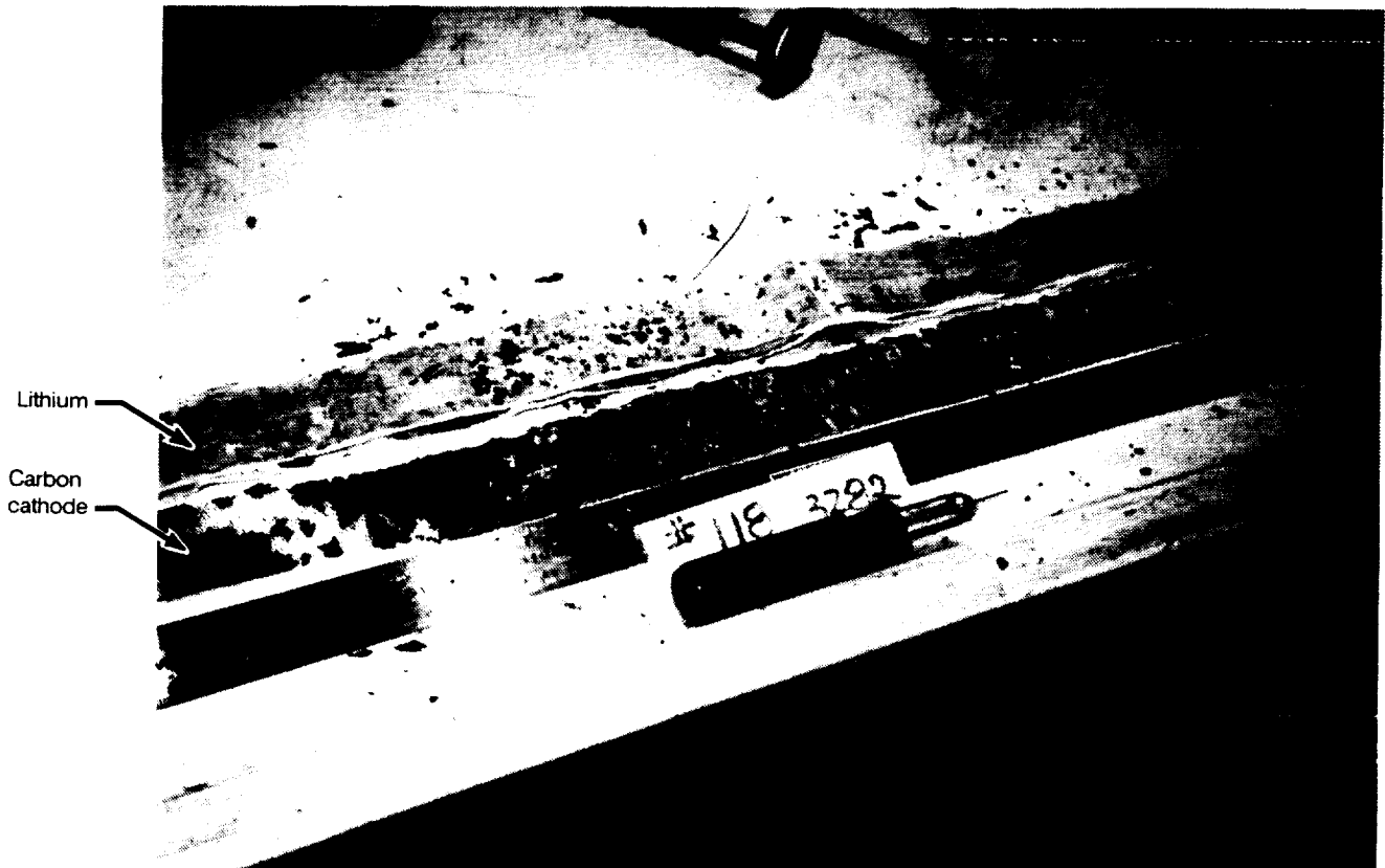
\text{LiSO}_2 Cell Components – Flight Battery With a 35% State of Charge
