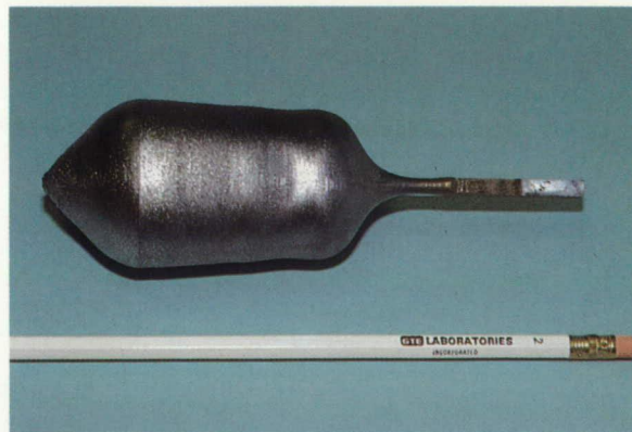
An Earth-grown gallium arsenide crystal seen next to a pencil for comparison
