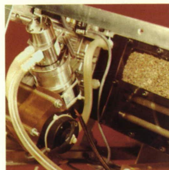
The Astroculture™ hardware consists of fluid pumps, fluid delivery and recovery tubes, and rooting matrixes. While several experiments have been performed on growing plants, Astroculture™ is the first attempt to develop a system for the precise watering and nutrient feeding of plants in the microgravity environment, where normal methods do not work effectively.
