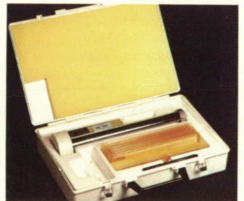
The Microbial Air Sampler will be used to determine the growth of fungi and bacteria over the course of USML-1's 13-day mission.
