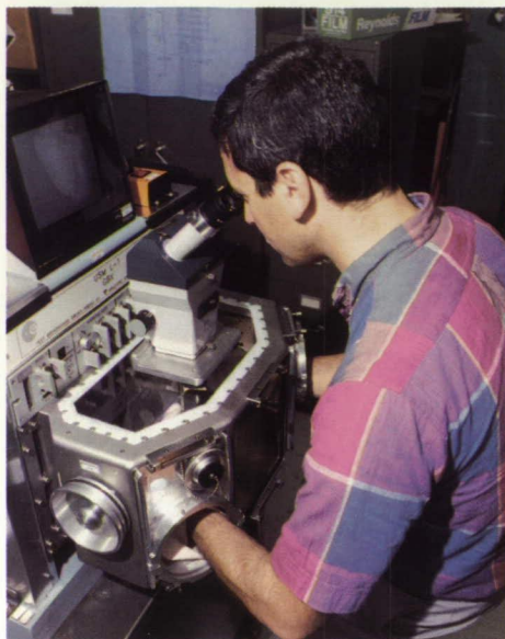
Payload Specialist Dr. Lawrence DeLucas tests a microscope for USML-1 on the engineering mockup of the Glovebox
