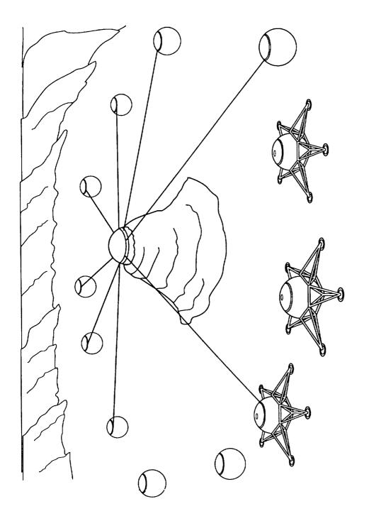
observation to maintain the equality of optical paths without the need for delay lines. Shown here based implementation in the coming years. The telescopes move in two dimensions during the are telescopes equipped with six robotic legs, like insects, and similarly able to move smoothly Figure 1: Lunar version of the Optical Very Large Array, which is studied for groundunder control of a laser metrology system.
