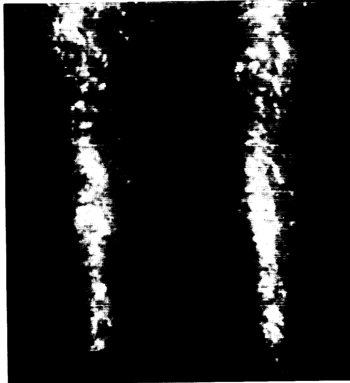
Figure 5. Two single-shot PLIF images of OH in the engine exhaust plume, obtained by pumping the (3,0) band.
