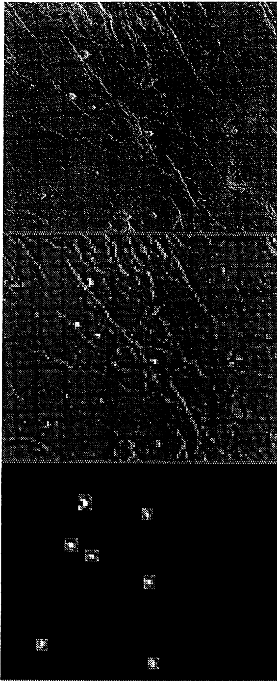
Fig. 1. Original Magellan SAR data (top), bandpass filtered version of same (center), and detected regions of interest (at 1/4 resolution) (bottom).
