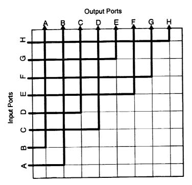
For near term applications in backend networking for supercomputers or attachment of peripherals, single stage switches with four to thirty-two port pairs are probably adequate. However, the limits of board to board connector technology means that we are rapidly approaching the limits of current switch architecture. Therefor, requirements which dictate greater HiPPI connectivity will probably use multistage switches constructed by cascading existing switches.
