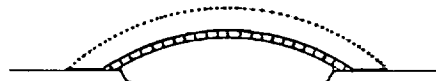
4. Alternative pressurized enclosure using hermetic membrane applied to inner surface of shield
