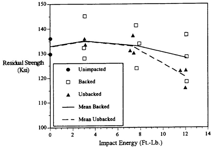
Figure 1. Plot of residual tensile strength versus impact energy for backed and unbacked specimens.
