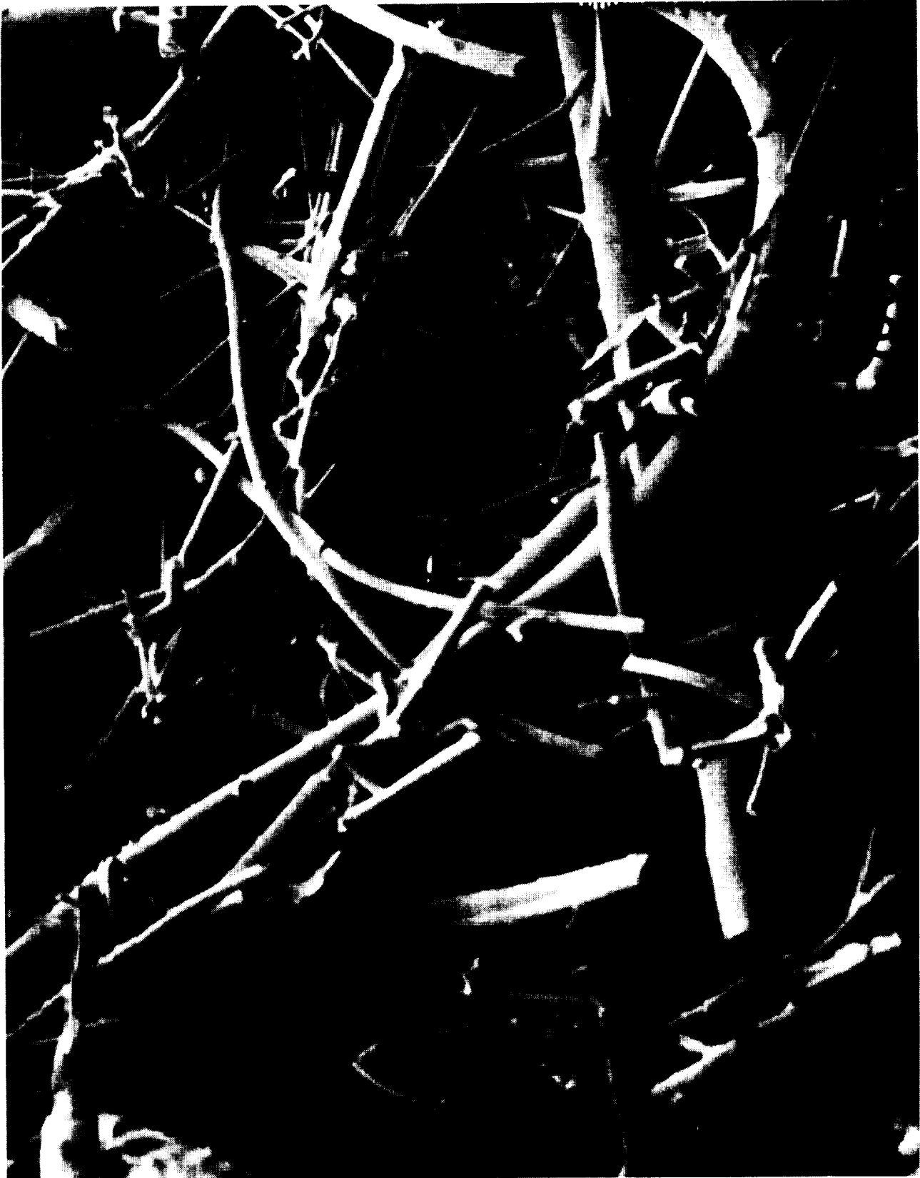
Fig. 1b Micrograph of FRCI-12 Surface Parallel to the Mold Line.
