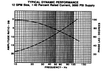
Graph 2. Servo-valve Time-Varying Response
