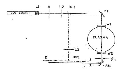
A schematic diagram for small angle  $CO_2$  laser scattering from a plasma. A rotating mirror RM scans the scattered radiation S at angle  $\phi_B$  to be coincident with the LO beam at BS2 and detector. The fluctuation of wavelength  $\lambda$  is determined from  $\phi_B = 2 \text{Sin}^{-1} \left( \lambda_o / 2 \lambda \right)$
