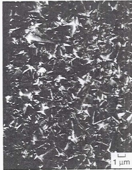
(b) Medium-grain (1100 nm) diamond film on (100) Si substrate; surface roughness R_{rms} = 63 nm.
