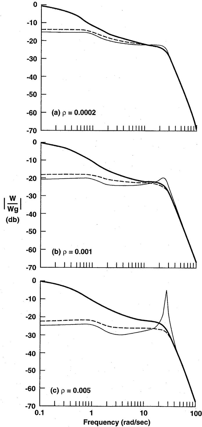
Figure 22. Effect of rotor state feedback on gust response: frequency response of vertical velocity to vertical gust input.
