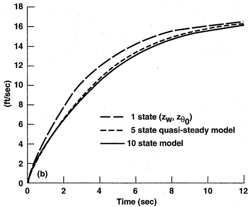
Figure 14a). Comparison of rpm responses to step (1 deg) collective input, b) comparison of rate-of-climb responses to step (1 deg) collective input.
