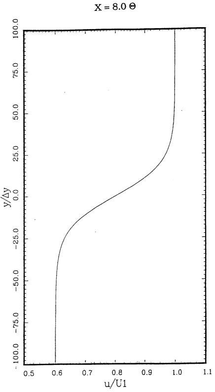
solid line: Boundary layer approximation for mean flow dot line: Parabolized Navie-Stokes approximation for mean flow (  $\Theta{=}40\Delta y$  )
