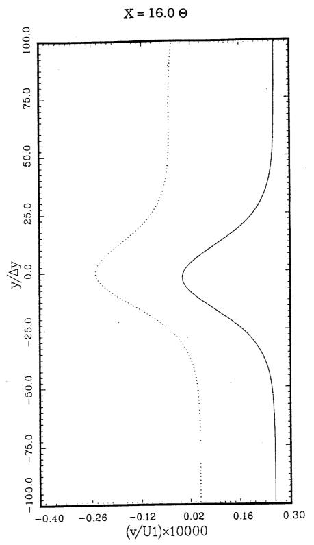
solid line: Boundary layer approximation for mean flow dot line: Parabolized Navie-Stokes approximation for mean flow (  $\Theta{=}40\Delta y$  )
