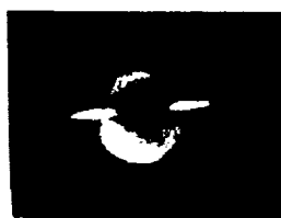
Figure 5.--Sequence of images showing the flame behavior just prior to, during and after what appears to be disruption of a droplet initially composed only of n-heptane. Times are after the ignition spark. For a scale reference, the visible flame diameter at 0.324 sec is about 4.7 mm (measured perpendicular to the fiber).
