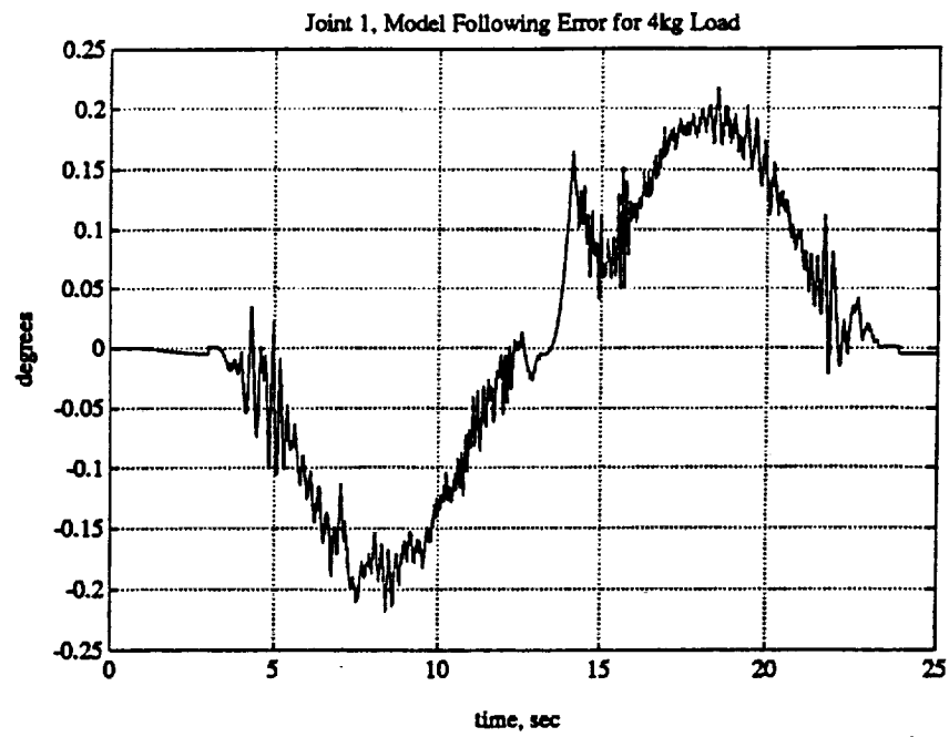
Figure 9.20: Joint 1 Dynamic Load Model Following Error for 4kg Load
