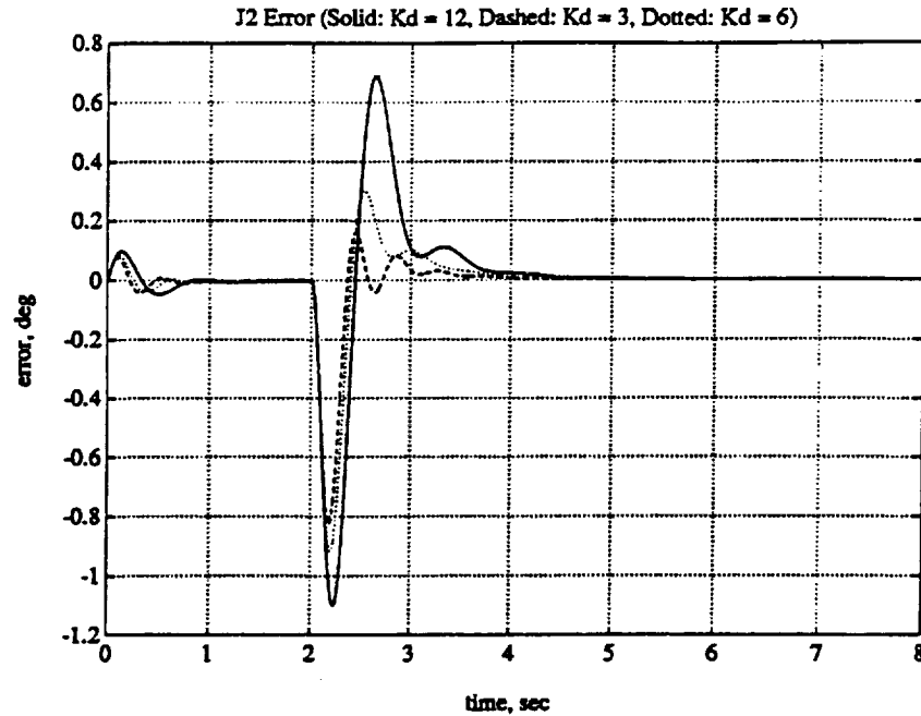
Figure 5.19: Effects of K_d in feed-forward on Joint 2. (dotted) K_d = 6 , (solid) K_d = 12 , (dashed) K_d = 3
