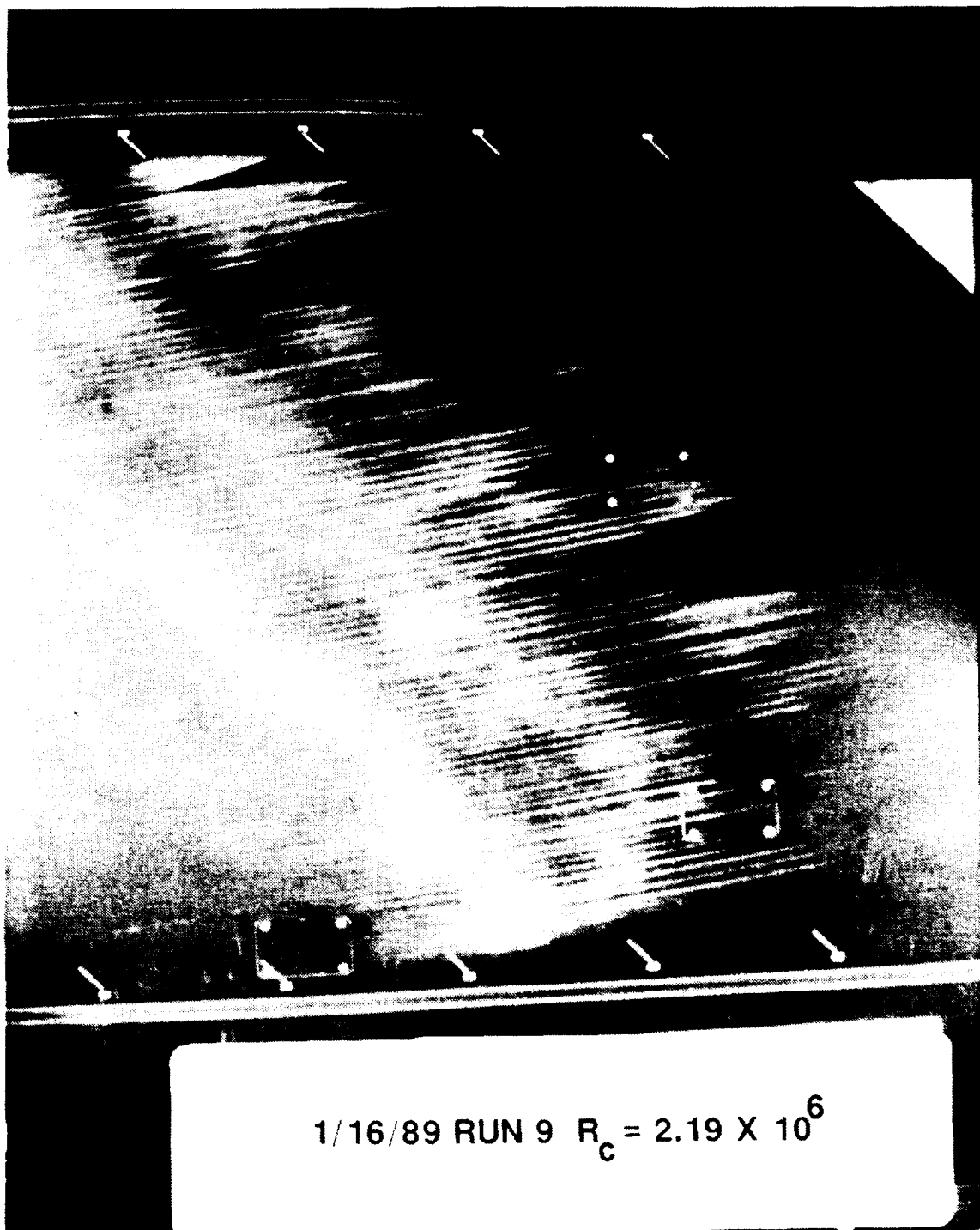
Figure 45. Naphthalene Flow Visualization, \alpha = -4^\circ , R_c = 2.19 \times 10^6 .
