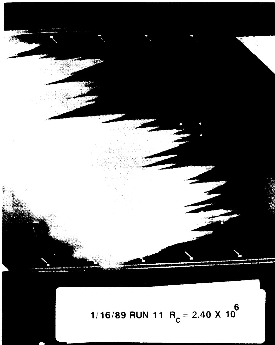
Figure 46. Naphthalene Flow Visualization, \alpha = -4^\circ , R_c = 2.40 \times 10^6 .
