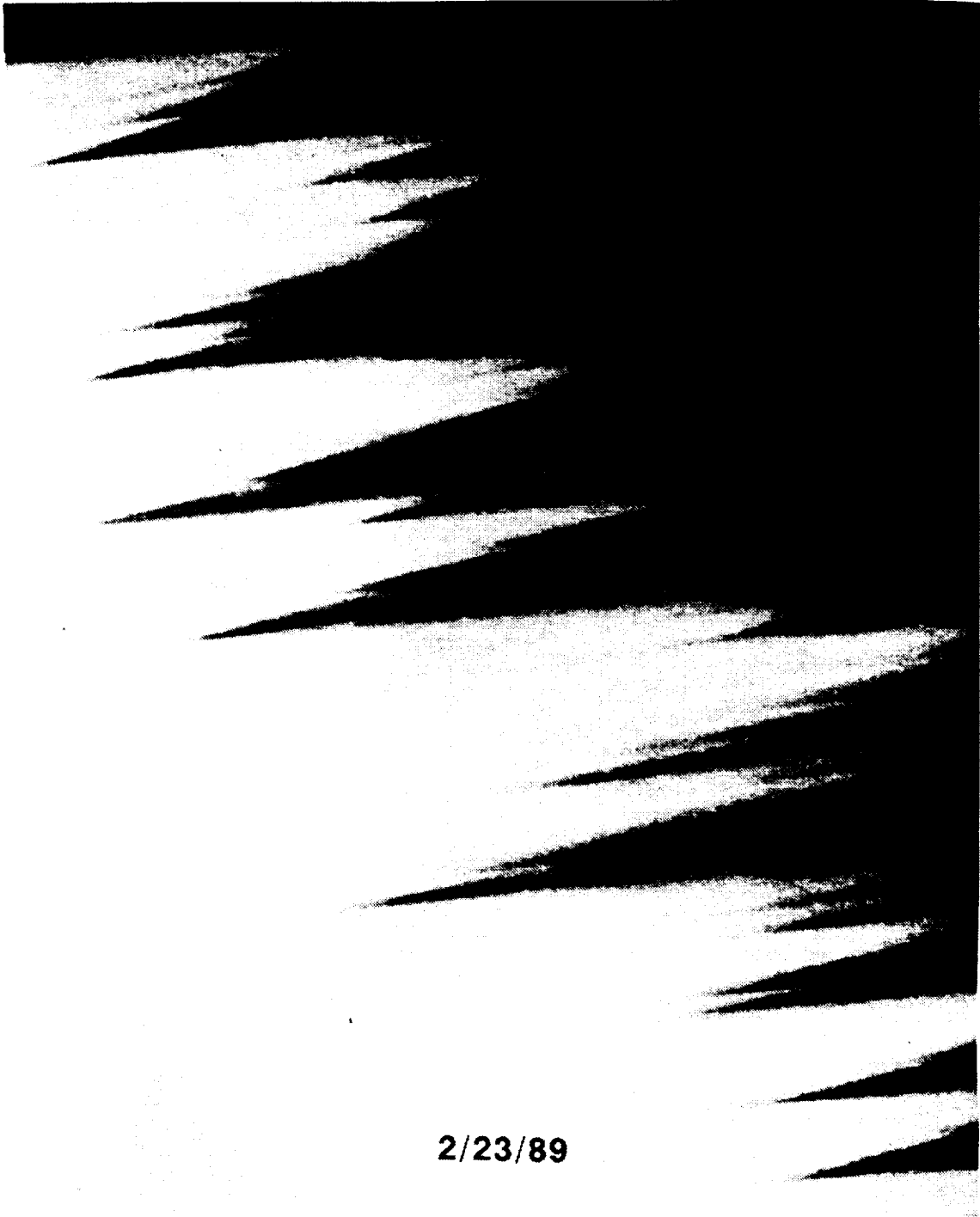
Figure 49. Naphthalene Flow Visualization Showing Vortex Tracks in the Turbulent Regions.
