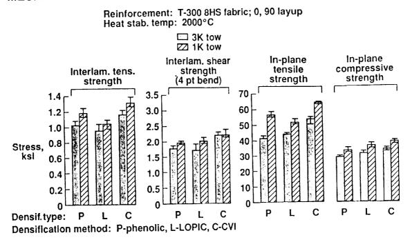
STRENGTH BENEFITS OF A CVI-DENSIFIED 3-D ORTHOGONAL CARBON-CARBON COMPOSITE
