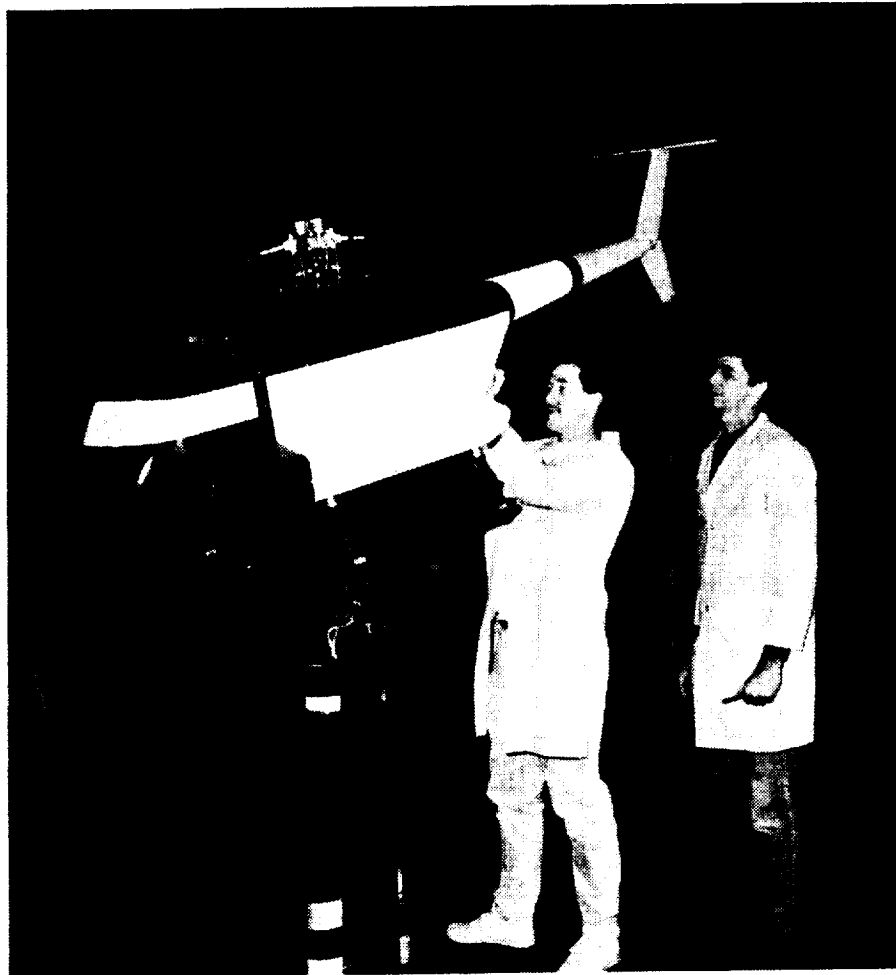
FIGURE 9: The Scaled Research Vehicle (FFRRV) In The NASA 14- by 22-Foot Tunnel.
