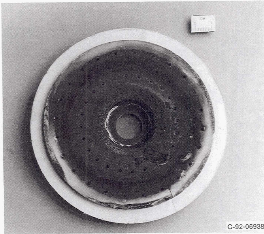
Figure 4.—Degradation of boron nitride insulator.
