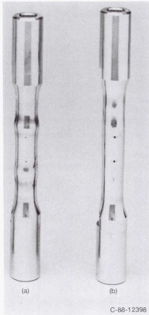
Figure 14.—Specimen barreling; (a) after 500 cycles, before improved techniques; (b) after 1100 cycles with improved control techniques.
