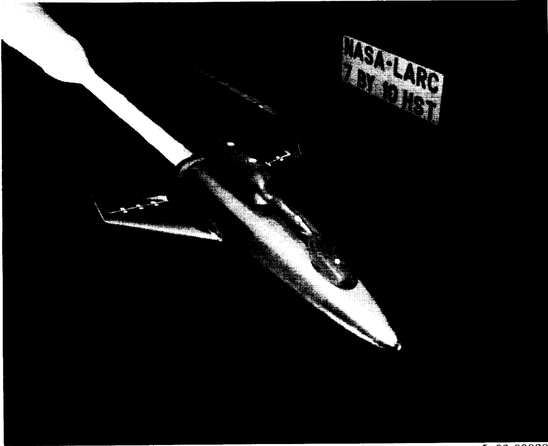
Figure 4. The AMLS orbiter model mounted in the Langley 7- by 10-Foot Tunnel.
