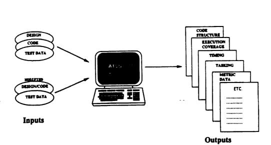
Ada Test & Verification System (ATVS) Analyses Capabilities
