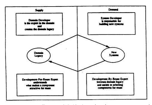
The continuous feedback loop between the supply and the demand side is the key to reuse
