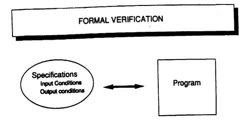
DEFINITION: Collection of techniques that apply the formality and rigor of mathematics to the task of proving the consistency between an algorithmic solution and a rigorous, complete specification of the intent (behavior) of the solution
