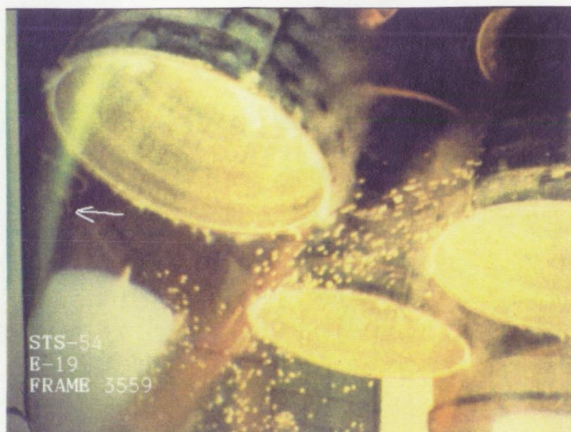
Figure 2.2.3 Green Streak in SSME #1 Plume
