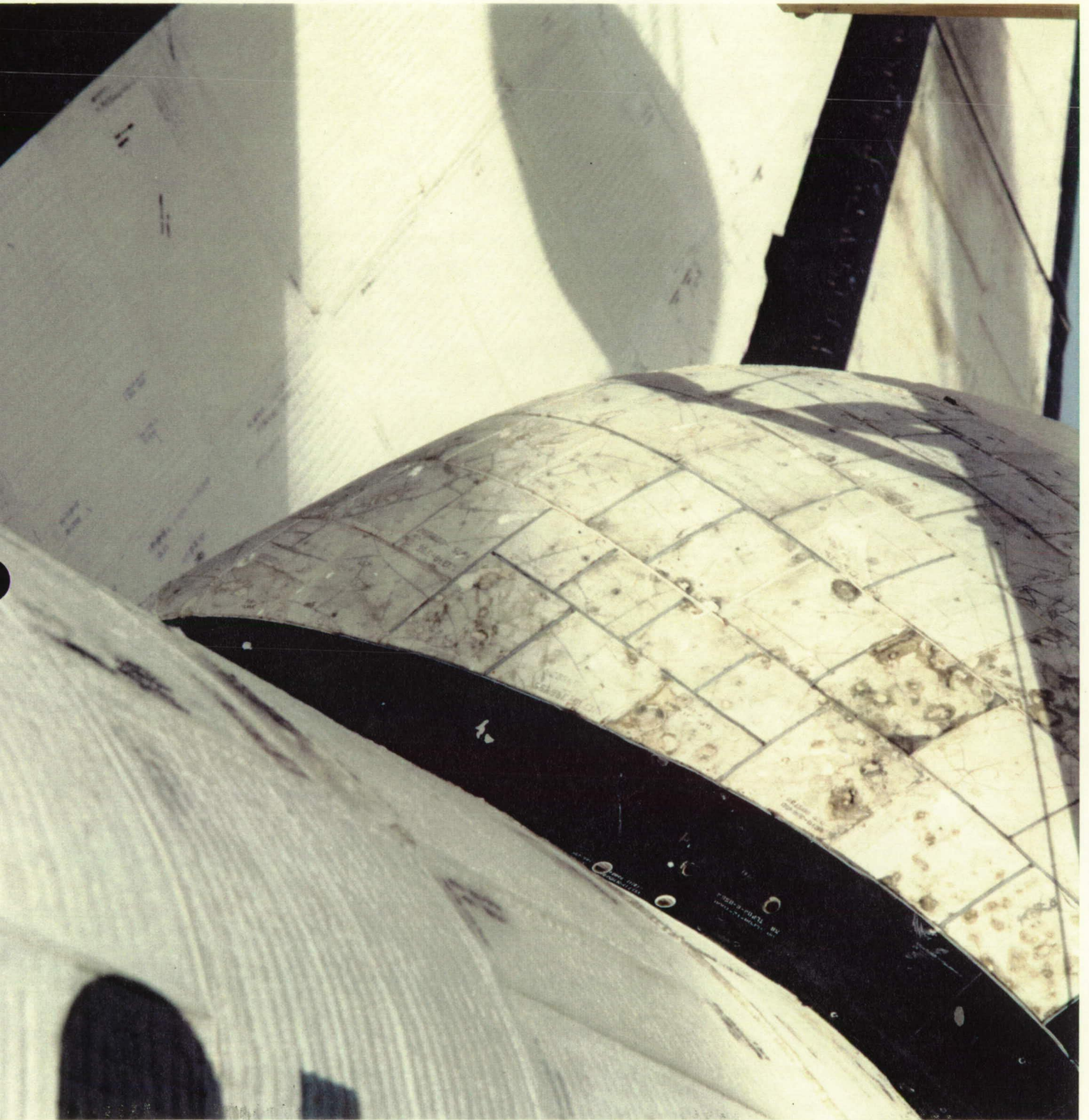
Tiles on the left OMS pod leading edge sustained more damage than usual. The cause of this damage is still undetermined.
