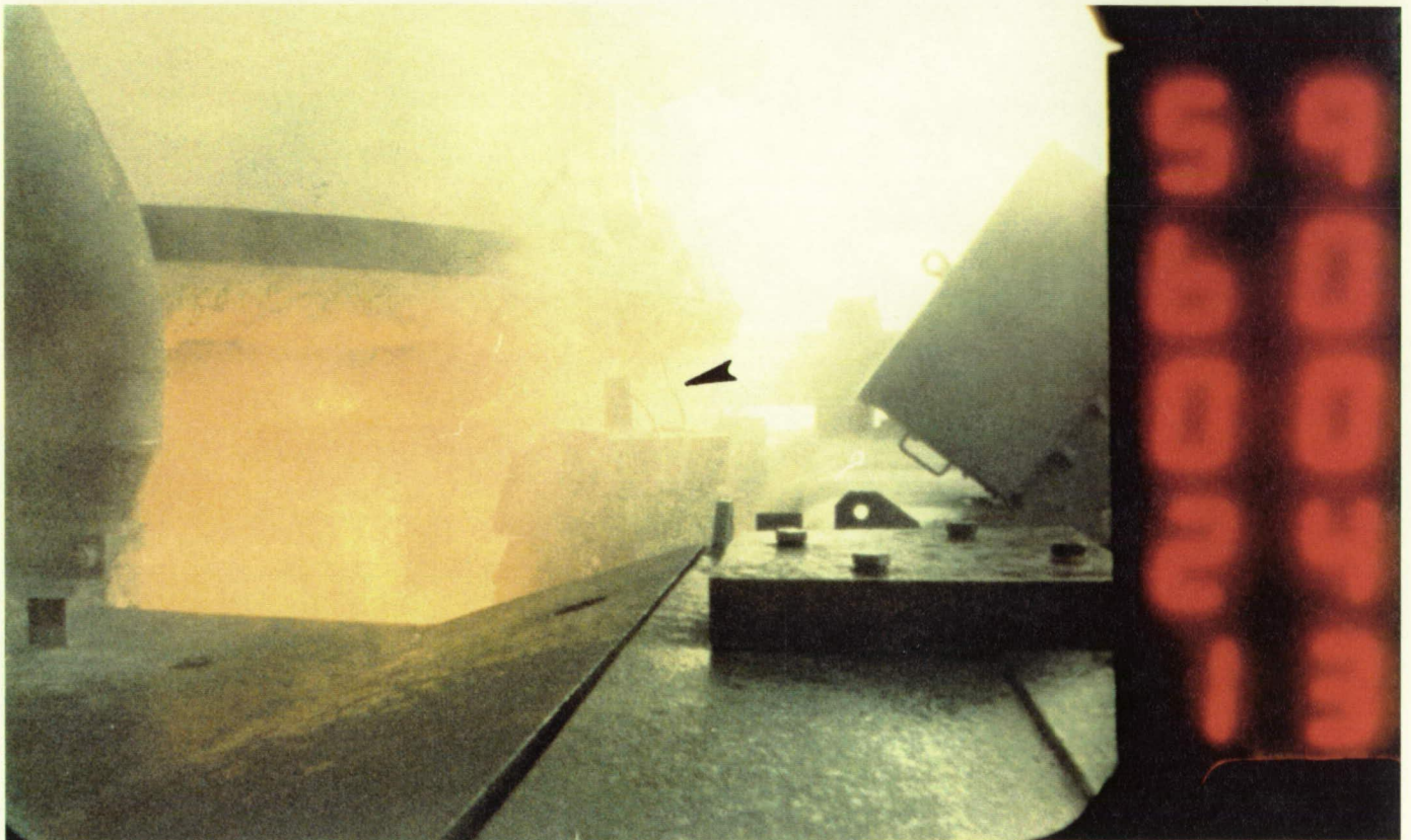
A stud hang-up occurred on HDP #1. One piece of ordnance debris fell from the DCS/stud hole into the HDP haunch area and may have been a frangible nut web.
