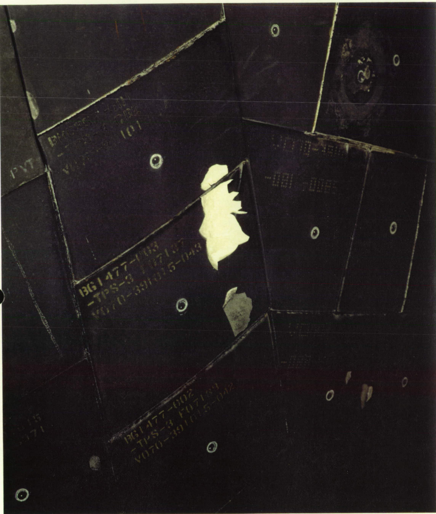
The Orbiter lower surface tiles sustained a total of 145 hits, of which 11 had a major dimension of 1-inch or greater. The majority of the tile damage occurred on the right side of the vehicle and was attributed to ice from the LO2 feedline.
