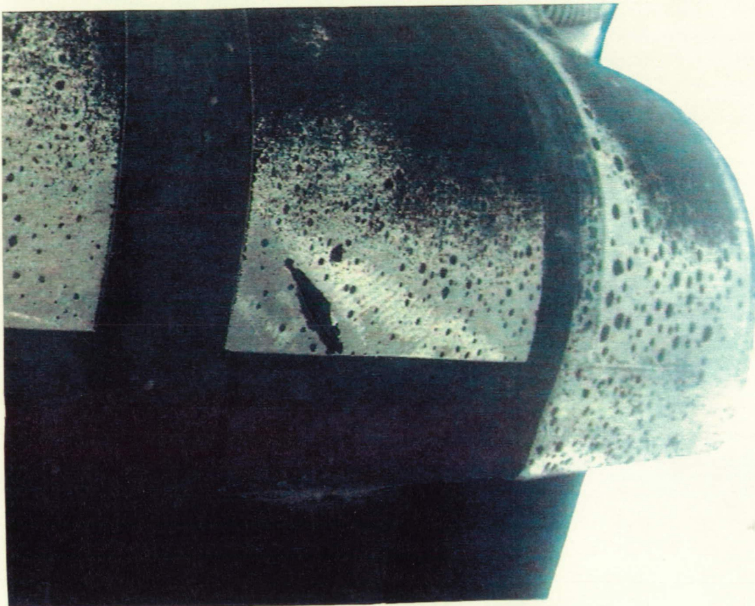
Figure 2.1.4a Elliptical Debris Strike on the RSRB Aft BSM Triple Motor Housing
