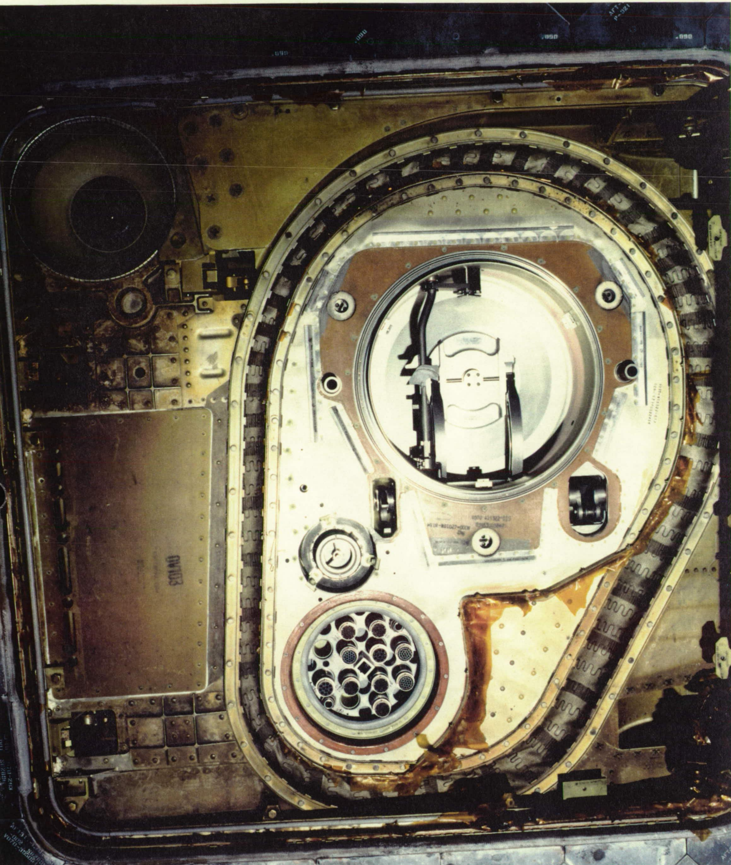
Overall view of the L02 ET/ORB umbilical. All separation ordnance devices functioned properly. No flight hardware was found on the runway below the umbilical when the ET door was opened.
