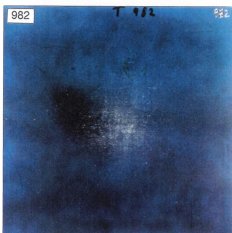
Figure 6. Witness-plate spray and damage patterns obtained by stacking an increased number of identical meshes; targets were impacted with soda-lime projectiles at constant velocity. The number in the upper left-hand corner of each frame is the experiment number (See Table 1 or Figure 3 for details). Note as the number of meshes increase from N=1 to N=10 that the degree of projectile comminution increases, while the amount of damage to the witness plate decreases. Experiments 813, 822 and 823 were described by Hörz et al. (1992a) and employed cylindrical witness plates, the reason for the ring-like termination of the spray patterns.
