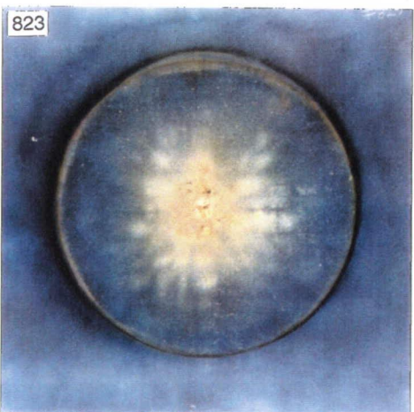
Figure 6. Witness-plate spray and damage patterns obtained by stacking an increased number of identical meshes; targets were impacted with soda-lime projectiles at constant velocity. The number in the upper left-hand corner of each frame is the experiment number (See Table 1 or Figure 3 for details). Note as the number of meshes increase from N=1 to N=10 that the degree of projectile comminution increases, while the amount of damage to the witness plate decreases. Experiments 813, 822 and 823 were described by Hörz et al. (1992a) and employed cylindrical witness plates, the reason for the ring-like termination of the spray patterns.
