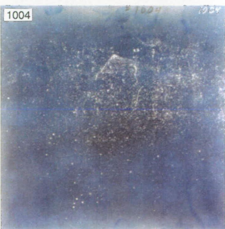
Figure 12. Illustrates the results of impacts at 2 and 5.9 km/s into mixed-mesh stacks; each stack consisted of a different number of meshes of very different specific mass resulting in a wide range of total cumulative bumper mass (SM). It is clear that more fragments and mass exit the low-mass designs compared to the more massive, five-member stacks. Note that numerous bumper fragments must have reached the witness plates compared to the commercial mesh experiments (e.g., 990), indicating that more massive bumpers are not necessarily advantageous.
