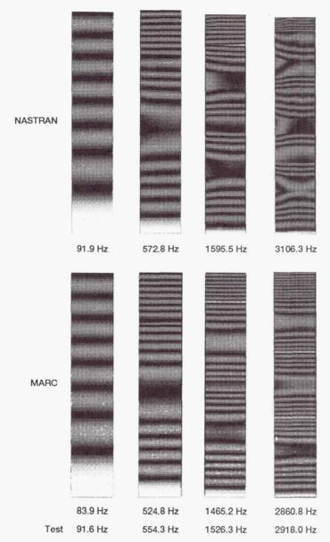
Figure 9.- Results for composite plate, form 1.
