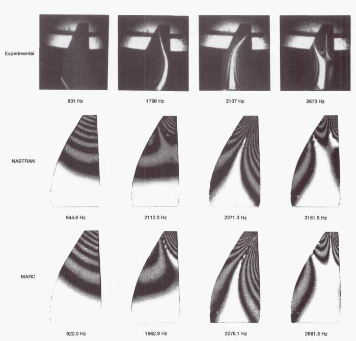
Figure 16. – Results for CM1 forward blade.
