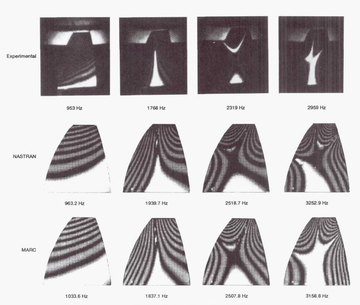
Figure 19. – Results for CM2 aft blade.
