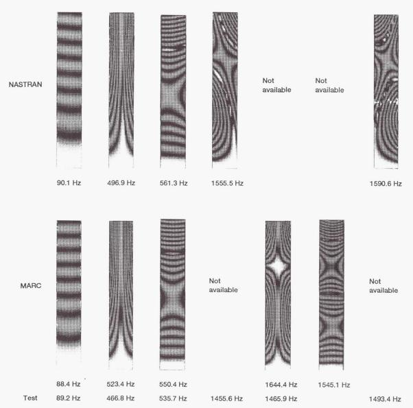
Figure 11. — Results for composite plate, form 3.
