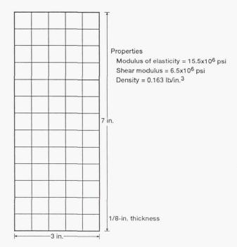
Figure 2. - Finite element model of flat plate.
