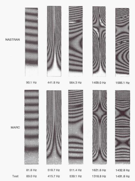
Figure 10. – Results for composite plate, form 2.
