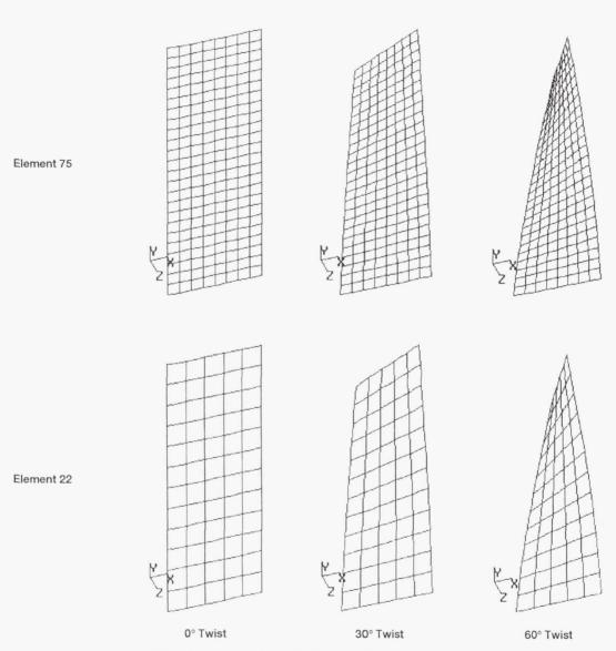
Figure 5. - Twisted plate study; MARC finite element models.
