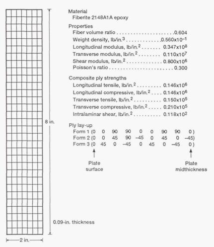
Figure 8. – Composite flat plate model, forms 1, 2, and 3.
