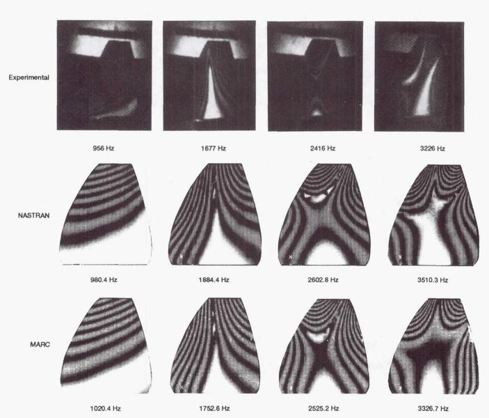
Figure 18. – Results for CM2 forward blade.
