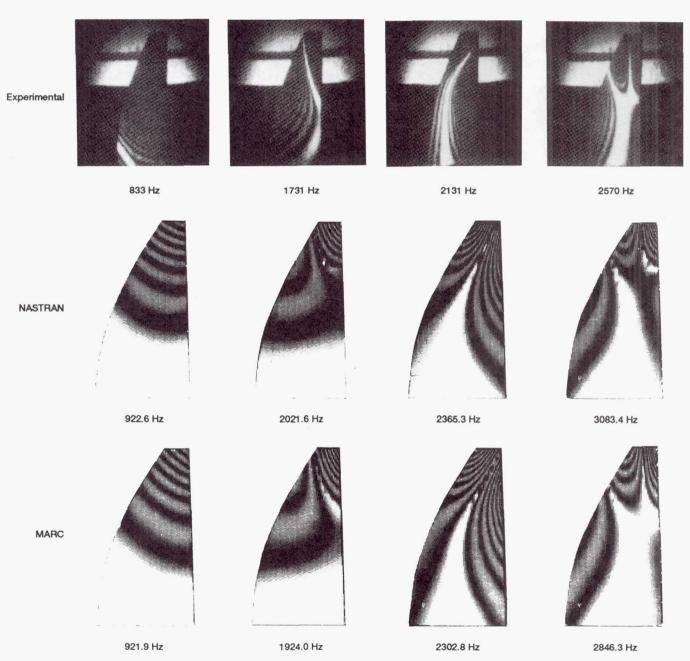
Figure 17. – Results for CM1 aft blade.
