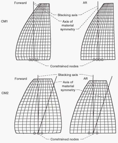
Figure 15. - Composite blade finite element models.
