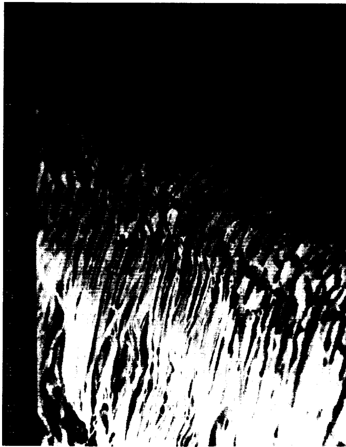
Figure 8. SEM of the edge of an FEP thermal control blanket recovered from the trailing edge of LDEF (at a magnification of 500).
