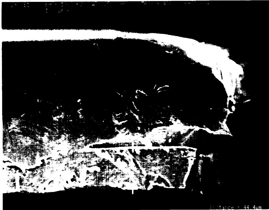
Figure 1. SEM of a control sample of an FEP thermal blanket, viewed at the edge (at a magnification of 400), showing the laminate structure of the bulk material.
