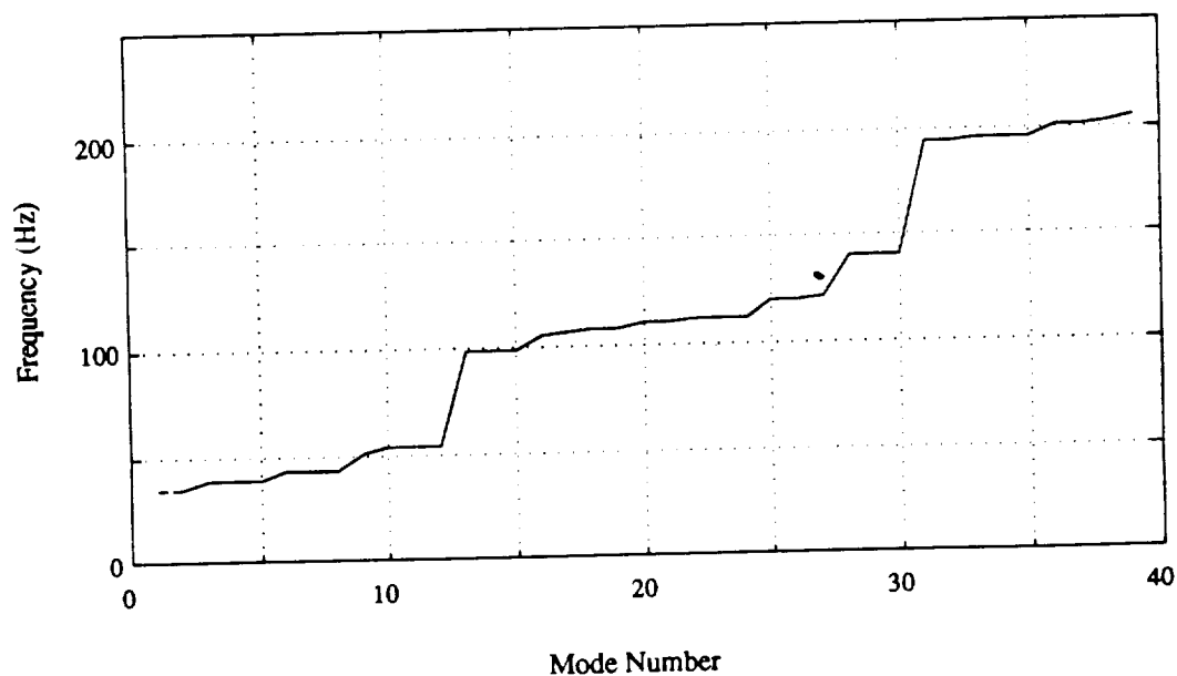
Figure 12: Frequency Distribution of First 39 Finite Element Modes
